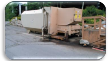
Dumpster leaking directly into a storm sewer
